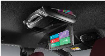
ENTERTAINMENT SYSTEM WITH ROOF MONITOR 5
