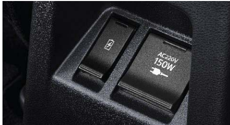
AC POWER OUTLET 220V/150W 1
